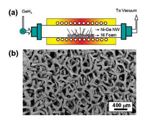
Figure 1. (a) Schematic diagram highlighting the CVD reaction of GeH<sub>4</sub> with a porous Ni foam substrate to form nickel germanide NWs. (b) Low-magnification scanning electron microscopy (SEM) image of the porous Ni substrate before reaction.
