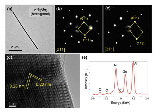
Figure 5. Structural characterization of the annealed nickel germanide NWs with hexagonal  $\varepsilon$ -Ni<sub>5</sub>Ge<sub>3</sub> phase. (a) Low-magnification TEM image; ED patterns taken from the (b) [211] and (c) [311] zone axes; (d) HRTEM image; and (e) EDS spectrum of the  $\varepsilon$ -Ni<sub>5</sub>Ge<sub>3</sub> NWs.
