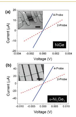
Figure 7. *I–V* characteristics (two-probe and four-probe) of representative (a) NiGe and (b)  $\varepsilon$ -Ni<sub>5</sub>Ge<sub>3</sub> NW devices. Inset shows representative SEM images of the NW devices. Scale bars are 2  $\mu$ m.
