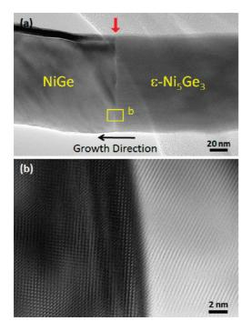
Figure 6. (a) TEM image of a heterostructured  $\epsilon$ -Ni<sub>5</sub>Ge<sub>3</sub>/NiGe NW. The interface is indicated by a red arrow. (b) HRTEM image of the  $\epsilon$ -Ni<sub>5</sub>Ge<sub>3</sub>/NiGe interfacial region.
