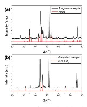
Figure 4. XRD patterns from the samples (a) before and (b) after annealing. The red lines indicate the standard diffraction peaks for (a) orthorhombic NiGe and (b) hexagonal  $\epsilon$ -Ni<sub>5</sub>Ge<sub>3</sub> phases. The completely indexed XRD patterns are shown in Supporting Information.
