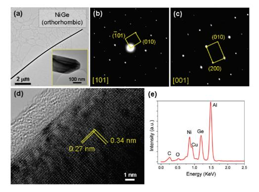
Figure 3. Structural characterizations of the as-grown nickel germanide NWs with orthorhombic NiGe phase. (a) Low-magnification TEM image (inset is a typical magnified view of NW tip), ED patterns taken along (b) [101] and (c) [001] zone axes, (d) HRTEM image and (e) EDS spectrum of the NiGe NWs.
